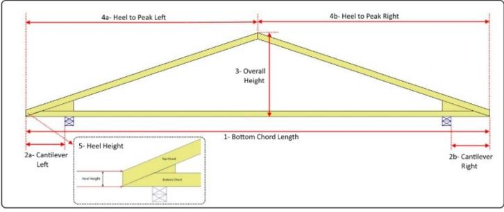
To match trusses to an existing trussed roof, fill in the following information for an accurate fit. Note: The chords do not have to be the same size (2x4,2x6, etc.) for the trusses to match.
