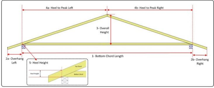
To match trusses to an existing trussed roof, fill in the following information for an accurate fit. Note: The chords do not have to be the same size (2x4,2x6, etc.) for the trusses to match.
